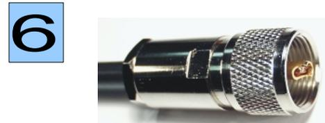
The prepared cable tail has to be carefully inserted into the housing until stop. Tighten the clamping nut finger tight with two open-ended spanners 16 mm.
