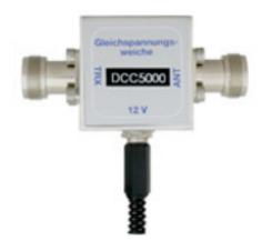
The remote powering coupler DCC 5000 is used for remote feeding of amplifiers and converters over the coaxial cable. The HF-oriented design and use of a ceramic printed board guarantee very low losses and excellent HF-matching.
