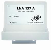
The GaAs-FET-Mast preamplifier LNA 137 A improves reception of low earth orbiting weather satellites in the 137 MHz range. The used GaAs-FETs in the input stage ensure a very low noise figure and high amplification as well. The mast preamplifier is equipped with an UV-resistant, weatherproof housing and N sockets. Hot galvanized clamps and mounting material made of V2A are part of the delivery.
