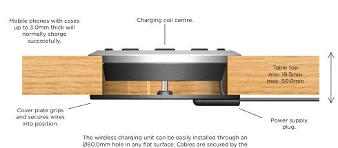
retaining plate completing the installation.
