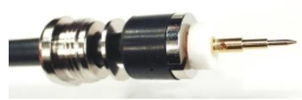
Put the Teflon washer over the inner conductor. Attach the inner pin and solder carefully through the small hole.
