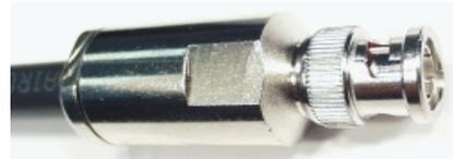
The prepared cable tail has to be inserted into the housing until stop. Tighten the clamping nut finger tight with two open-ended spanners 16 mm. A small split should remain visible between clamping nut and connector housing.
