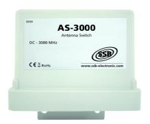
The antenna switch **AS-3000** is an electrically operated switch for two antennas. The unit is built into a weatherproof housing with mast mount. The switch is equipped with a highly loadable power relay, which is built into a weatherproof UV-resistant plastic housing. The lower part consists of a solid aluminiumangle mit zinc plated clamps for installation at the mast. The switch is suitable from DC to 3000 MHz.
